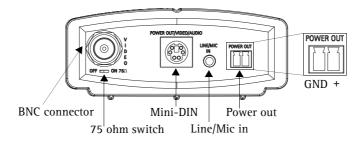
Power out - Used to power a camera or other auxiliary equipment 12V DC, max. load 5W (420mA)
