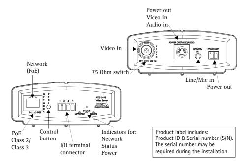
Network Connector - The Video Server connects to the network via a standard, shielded network cable, and automatically detects the speed of the local network segment (10BaseT/100BaseTX Ethernet). PoE Supported.
